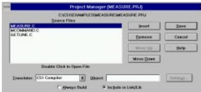
The Project Manager dialog box shows the source files that compose the MEASURE project. There are three source files in this project.
