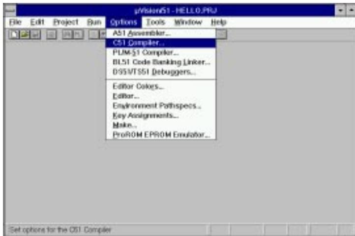
The menu bar provides you with access to menus for file operations, editor operations, project maintenance, external program execution (such as running the dScope debugger/simulator or another program), development tool option settings, window selection and manipulation, and on-line help.
