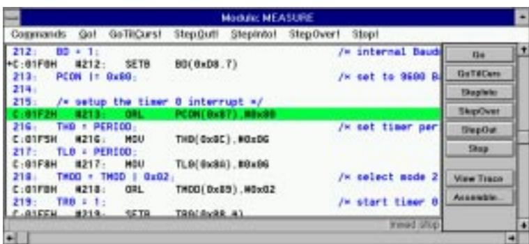
The debug window shows intermixed source and assembly lines.
