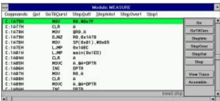
The StepInto button lets you single-step through your application and into function calls. Click on the StepInto button a few more times to get to the loop which clears the on-chip data space of the CPU.
