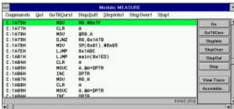
The StepInto button lets you single-step through your application and into function calls. Click on the StepInto button a few more times to get to the loop which clears the on-chip data space of the CPU.
