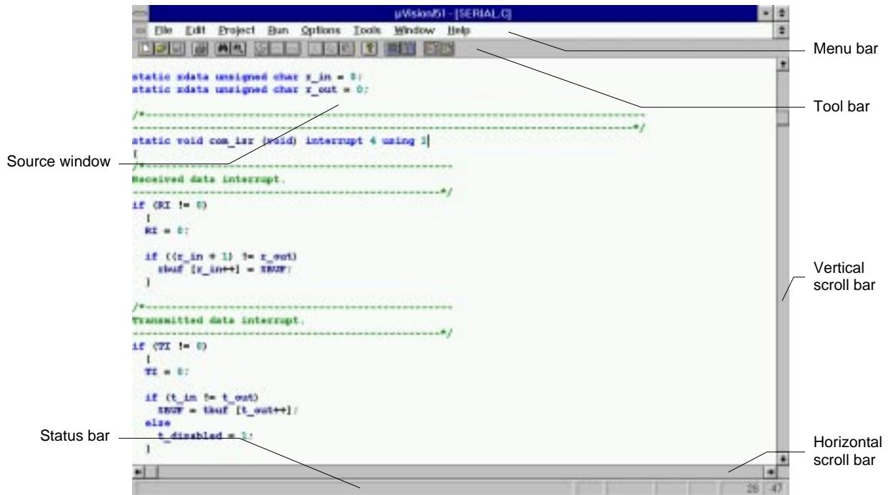
You can quickly access many of the features of µVision using the buttons on the tool bar.
