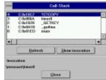
You can display the caller of a function by selecting the function from the list. Then, you can use the Show invocation button to display the function call in the debug window.
