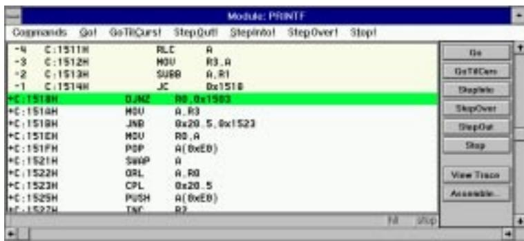
The upper portion of the debug window shows the trace history. The lower portion of the debug window shows instructions from the program counter. The program counter line is the delimiter between the trace history and instructions not yet executed.
