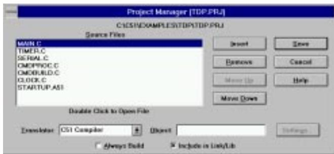
All aspects of a project are saved in a project file. The project file includes: the source files that make up the target program; the compiler, assembler, and linker command line options; the debugger and simulator options; and the make facility options.
