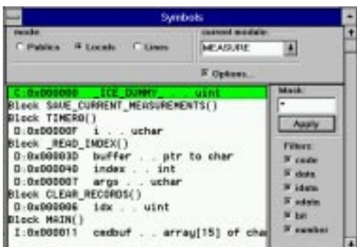
dScope supports the drag and drop feature of Windows and lets you access the symbols this way. Use the mouse to drag and drop the **idx** symbol from the symbol browser window to the command window. The fully qualified symbol
