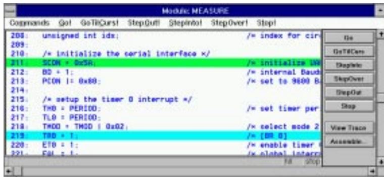
Click on the Go button and dScope starts execution from the current program counter and stops when the breakpoint is reached. To remove a breakpoint, double-click on the line containing the breakpoint.
