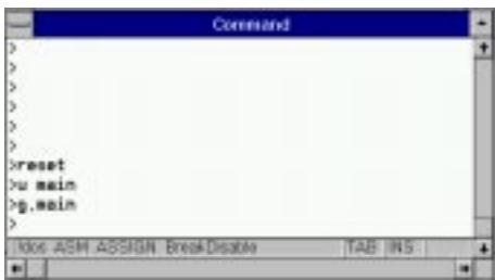
You can interactively display and change variables, registers, and memory locations from the command window. You can also enter assembly code to patch or test parts of your program.
