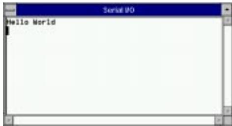
After HELLO outputs “Hello World,” it begins executing an endless loop. To halt execution, click on the Stop button in the debug window or type **Ctrl+C**. After you have halted program execution, you may type **exit** to leave the dScope debugger.
