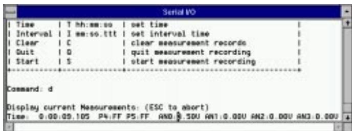
The serial window displays what you would see on a dumb terminal connected to the 8051's serial port.
